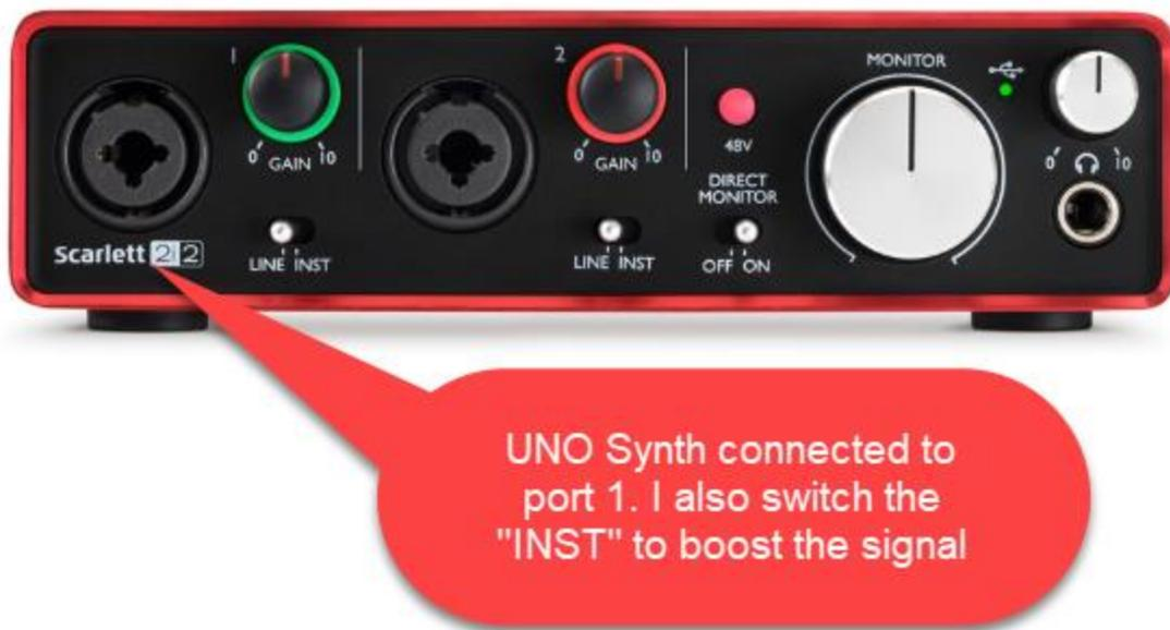
Remember to switch the button from LINE to INST and control the gain so the audible sound doesn't distort or clip the sound from the UNO Synth.
