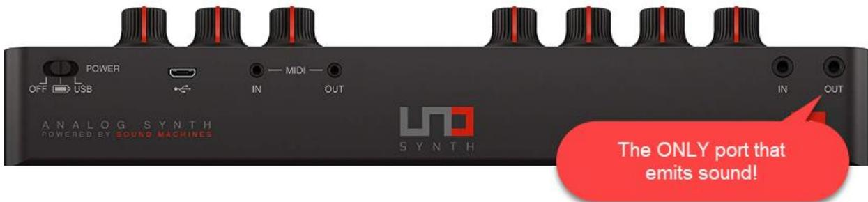
The port above should be connected to your audio interface's audio ports
